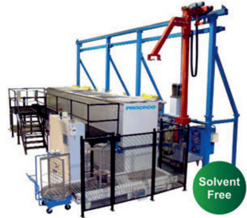
Ultrasonic immersion degreasing
