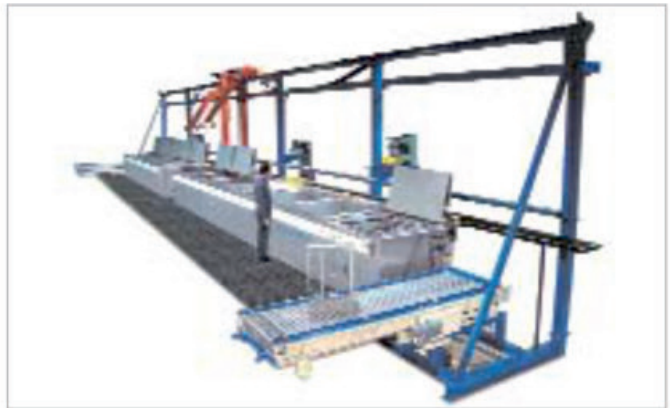
12-stage automated fluorescent penetrant inspection FPI and degreasing tank line
