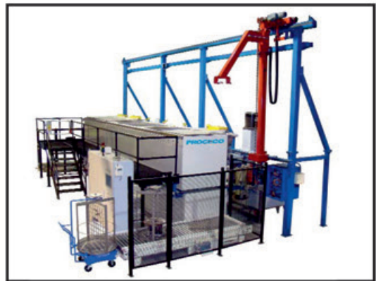
6-stage automated ultrasonic immersion degreasing line featuring automatic basket loading/unloading and convection drying.
