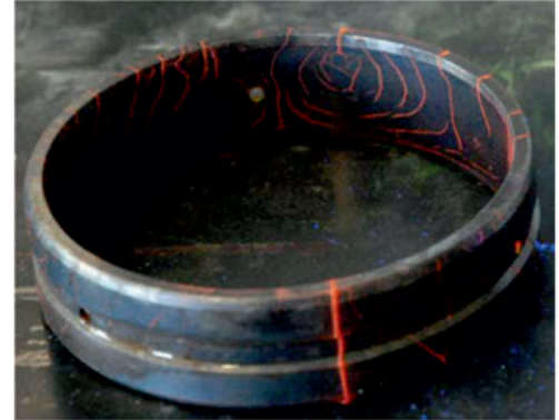
Crack indication resulted from application of the water-based suspension prepared by use of MEF 515 dry concentrate.
