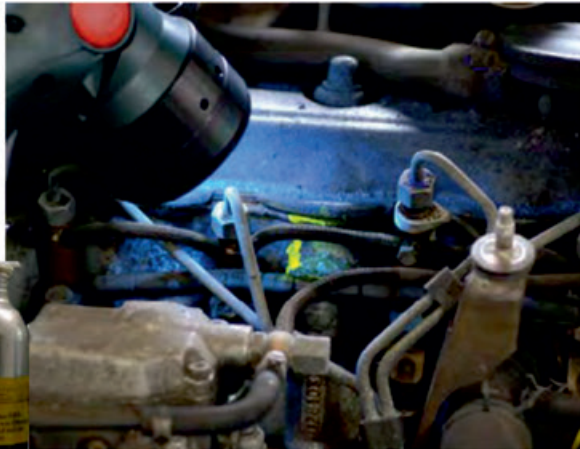
Leak detection in automobile engine by use of H 800 fluorescent concentrate
