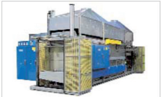
7-stage automated immersion line featuring power spray cleaning, deoxidizing, and automatic loading / unloading.
