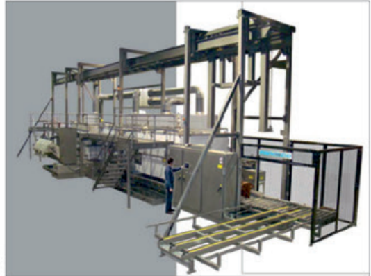
5-stage automated immersion line with cleaning and paint stripping of armored vehicle engine components
