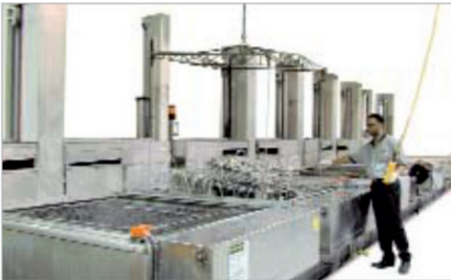
10-stage manual immersion line featuring pump / eductor agitation, degreasing and heat scale removal.
