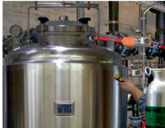
Detection of vessel depressurization by use of H 849 fluorescent concentrate
