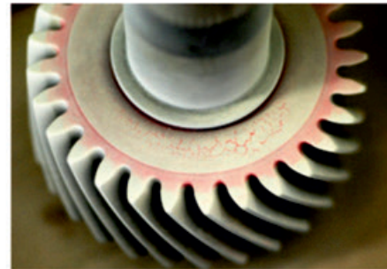
Defects indication resulted from contrast penetrant system application
