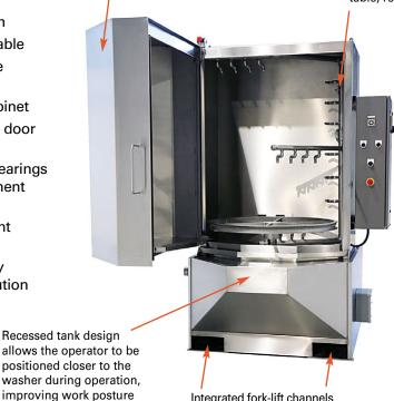
The C-shaped spray manifold sprays from the top, side and bottom of the rotating table, reaching all part surfaces.
